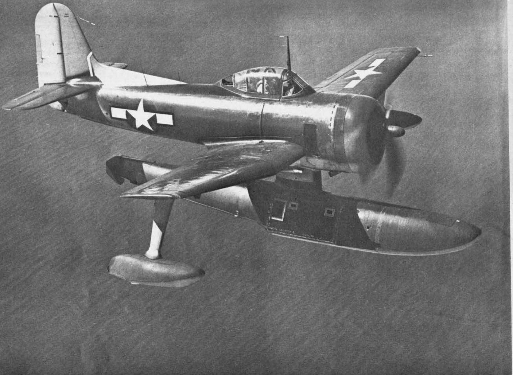
CURVED LINES OF SC-1'S FIN AND RUDDER CONTRAST WITH SQUARE LINES OF WING. NOSE IS HEAVY AND EGG-SHAPED LIKE THOSE OF F6F AND P-47
